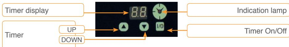
The timer indicates the baking time in minutes, from 0 to 99 minutes.
