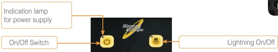
Before starting operation, you should press the on/off switch.
